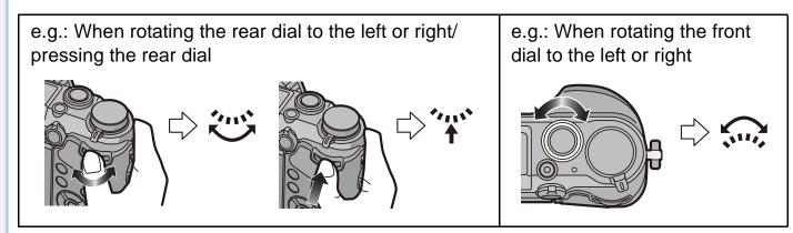
Allows you to set the aperture, shutter speed, and other settings when in P / A / S / M modes.
