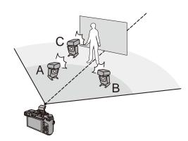
• In this placement example, flash C is placed to erase the shadow of the subject that flashes A and B will create.
